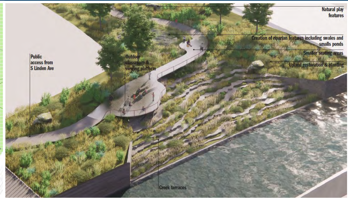
Incremental naturalising of the creek edge through the creation of creek terraces
